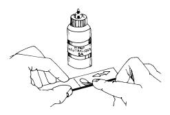
Now apply a liberal amount of Neutralizer 5A and scrub with a cotton-tipped applicator. With a single, slow wiping motion of a gauze sponge, carefully dry this surface. Do not wipe back and forth because this may allow contaminants to be redeposited on the cleaned surface.
