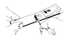
Apply a thin layer of adhesive to the gage bonding side and to the specimen. The adhesive film should be just thick enough to cover the gaging area without bubbles or voids. Approximately 0.002 in [0.08 mm] is typical on metal surfaces. Any lumps of unmixed adhesive should be removed before proceeding.
