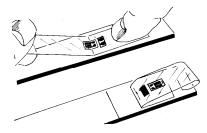
Lift one end of the tape at a shallow angle to surface (about 45 degrees) until the gage and terminal are free of the specimen surface. Tuck loose end of the tape under and press to surface so the gage lies flat with the bonding side exposed. Leave enough slack in the tape to allow a finger to be slipped behind the gage to support it while applying the adhesive (Step 7).
