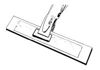
Either HSC-X spring clamps, as in, or deadweight can be used to apply pressure during the curing cycle. A clamping pressure of 10 to 30 psi [70 to 200 kN/m2] is recommended. Place clamped gage/specimen into a cool oven and raise temperature to the desired curing level at a rate of 5° to 20°F [3° to 11°C] per minute.
